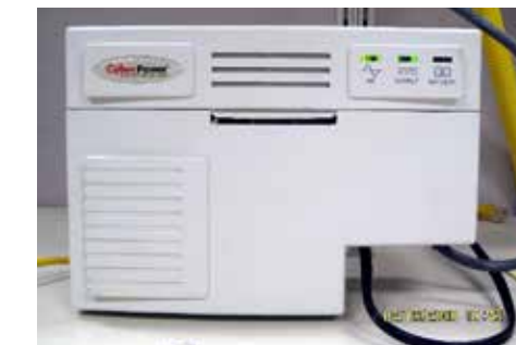
The picture to the left is a photo of a Cyber Power batter back up. This applies only to our members who are connected to the fiber optic cable.
